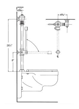
Valve is certified to be in compliance to the applicable sections of ASSE 1037 and ANSI/ASME 112.19.2
