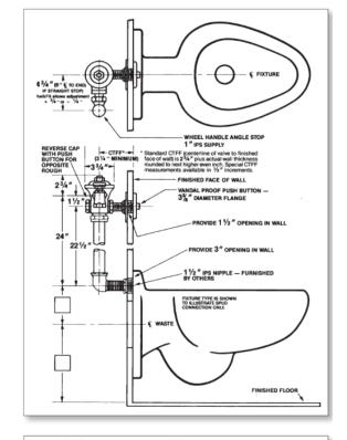
Recommended For: Penal or heavier duty installations where vandalism and abuse are common. No parts of valve can be removed from front face of wall. Access to rear of wall for future service of valve and vacuum breaker must be provided.
