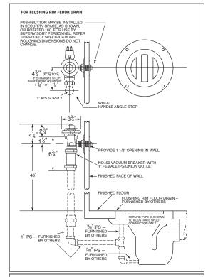
Recommended For: Facilities for disturbed inmates who are unwilling or unable to care for their own needs. No parts of valve can be removed from front face of wall. Pushbutton may be located as shown or rotated 180 for operation by attendant through wall of non-security area. In either case access to valve and vacuum breaker for future service must be provided.
