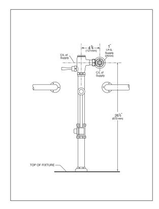
Valve is certified to be in compliance to the applicable sections of ASSE 1037 and ANSI/ASME 112.19.2
