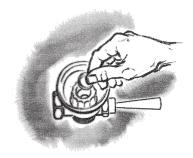
the flush valve, and replace the valve cover only. The flush valve has in effect been converted into an elbow in the line. If a syphon cannot be obtained under this condition, it will not be obtained until the pressure is increased.
