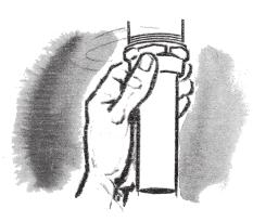
The Delany VB and flush connection are of unitized design and are coupled to the valve outlet in one operation. When making up the cowl nut to the valve outlet, a hand tight connection is sufficient. If further wrenching is done, use one quarter turn at most. The shoulder of the rubber sleeve in the vacuum breaker is its own gasket and will not leak if this light pressure is applied.
