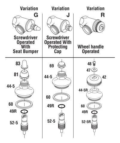
Type of operating mechanism must be specified for complete stops or bonnet assemblies. Select appropriate variation letter from chart above and suffix to assembly number. For example: 44-5A-J, 44-5A-G, etc. Choice of operating mechanisms does not change price of complete stops or partial assemblies above.
