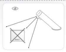
Check that there are no objects in front of the sensor after the battery replacement was completed.
