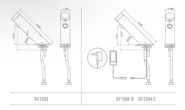
**Power Supply:** 9V battery or 9V transformer
